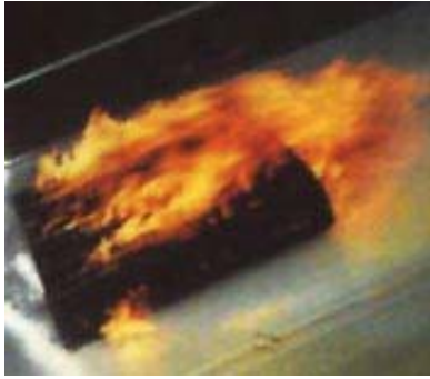
ASTM E-108 Burning Brand Test on Quadwall “Class A”
